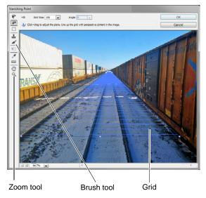
Figure 6 Perspective plane grid created
